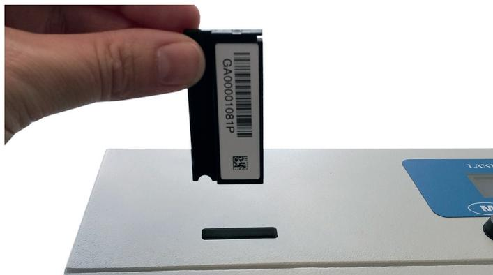
Positioning of a GA InLight dosimeter
