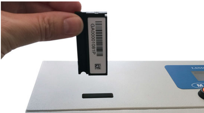
| Positioning of a GA InLight dosimeter
