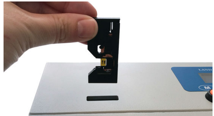
| Positioning a nanoDot in its adapter
